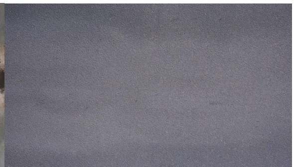
C1.1 火工后底漆冲砂 Sa2 1 / 2
